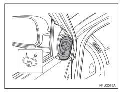
If your vehicle has this feature, the control for the power mirrors is located on the driver's side door trim.
